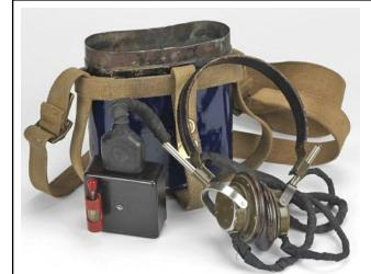
Detail view of the crystal receiver hidden in a modified pattern 37 water bottle.
